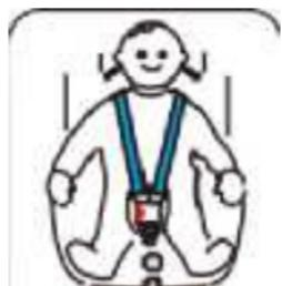
Pull the shoulder straps upwards to remove the whole harness then pull the adjuster strap until the harness is fully tightened (fig. left).
