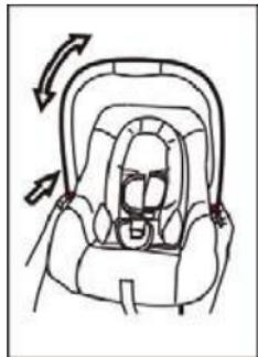
The handle for the baby car seat can be snapped into 4 stable positions. To adjust the handle, please press the red button of handle on both sides at the same time. Now it can be rotated.
